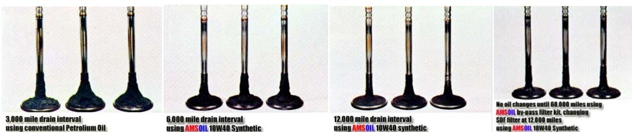
The short story? The synthetic oil provided protection of the test engines far beyond the normal 3,000-mile oil change interval. In fact, the engines run with synthetic oil for the full 60,000 mile showed less wear than did the group that had oil changes every 3000 miles.
